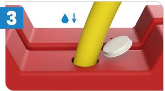
Insert a hose into the open filler hole, and begin filling the barrier. Adding water converts the Bison from a 35kg shell into a robust 400kg traffic barrier.
