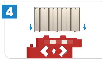
To add hoarding, lift the panel into the slot which runs along the top of the Bison. Line up the brackets on the panel with the holes on the barrier.
